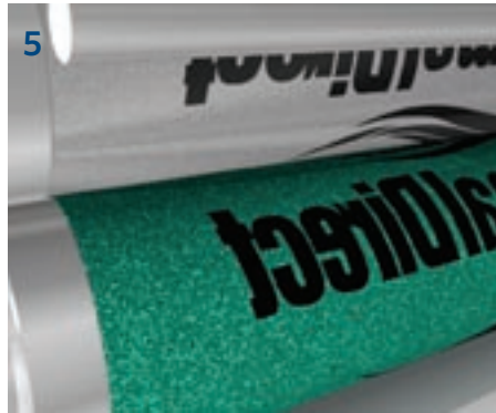
5 The fountain solution plus the ink tack ensure that the dissolving coating is transferred to the blanket, and so to the first few sheets.
